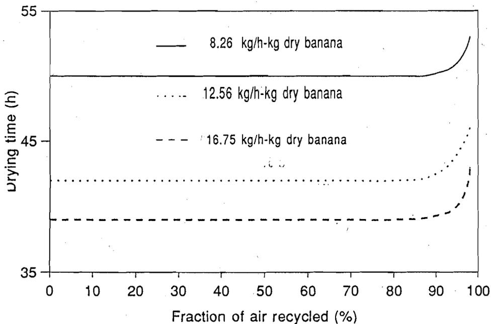
Fig. 9. Effect of fraction of air recycled on drying time at different specific mass flow rate (Temperature = 60°C).
