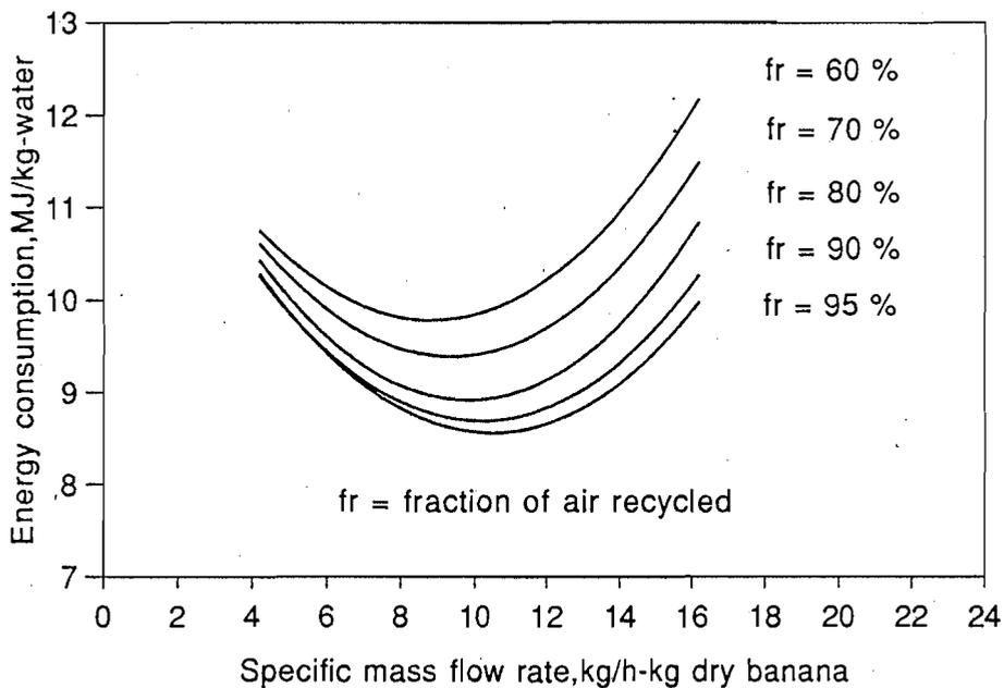
Fig. 8. Effect of specific mass flow rate on energy consumption at different fraction of air recycled (Temperature = 60°C).
